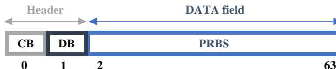
Figure 19: PRBS frames sent during the PRBS Alignment Sequence (PAS).
