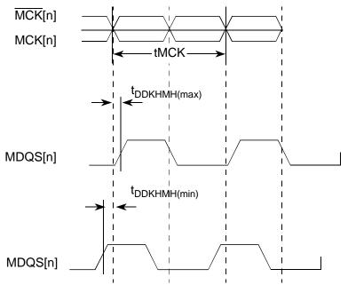
This figure shows the DDR3 and DDR3L SDRAM output timing diagram.
