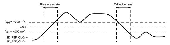
Figure 42. Single-ended measurement points for rise and fall time matching
