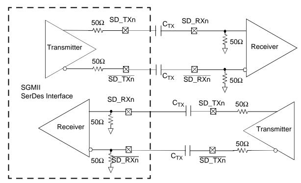
This figure shows the SGMII transmitter DC measurement circuit.
