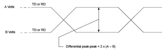
To illustrate these definitions using real values, consider the case of a CML (current mode logic) transmitter that has a common mode voltage of 2.25 V, and each of its outputs, TD and TD\_B, has a swing that goes between 2.5 V and 2.0 V. Using these values, the peak-to-peak voltage swing of the signals TD and TD\_B is 500 mV p-p. The differential output signal ranges between 500 mV and –500 mV. The peak differential voltage is 500 mV. The peak-to-peak differential voltage is 1000 mV p-p.
