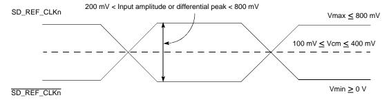
For an external AC-coupled connection, there is no common mode voltage requirement for the clock driver.
