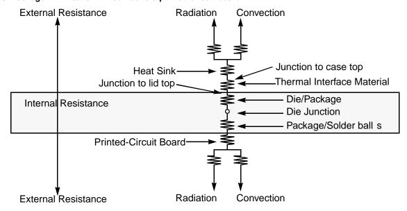
The heat sink removes most of the heat from the device. Heat generated on the active side of the chip is conducted through the silicon and through the heat sink attach material (or thermal interface material), and finally to the heat sink. The junction-to-case thermal resistance is low enough that the heat sink attach material and heat sink thermal resistance are the dominant terms.
