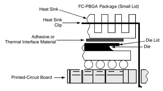
The system board designer can choose between several types of heat sinks to place on the device. There are several commercially-available thermal interfaces to choose from in the industry. Ultimately, the final selection of an appropriate heat sink depends on many factors, such as thermal performance at a given air velocity, spatial volume, mass, attachment method, assembly, and cost.
