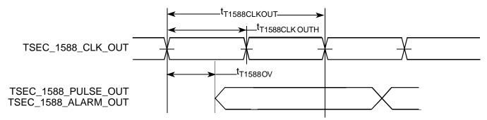
Note: The output delay is counted starting at the rising edge if tT1588CLKOUT is non-inverting. Otherwise, it is counted starting at the falling edge.
