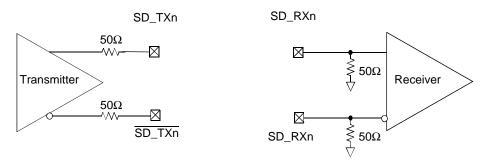
The DC and AC specification of SerDes data lanes are defined in each interface protocol section below based on the application usage:
