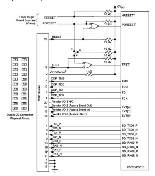
Figure 62. Aurora 22 pin connector duplex interface connection
