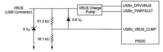
USB1\_DRVVBUS and USB1\_PWRFAULT are muxed on GPIO[4:5] pins, respectively. USB2\_DRVVBUS and USB2\_PWRFAULT are muxed on GPIO[6:7] pins, respectively. Setting the RCW[GPIO] bit selects USB functionality on the GPIO pins.
