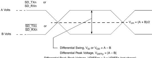
Differential Peak-Peak Voltage, VDIFFpp = 2 x VDIFFp (not shown)
