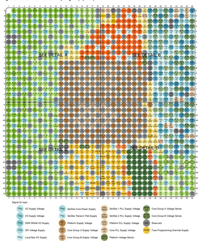
Figure 4. P5020–1295 BGA ball map diagram (detail view A)
