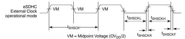
This figure provides the data and command input/output timing diagram.
