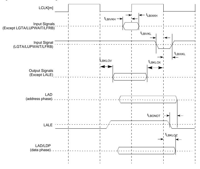
Figure 26 applies to all three controllers that eLBC supports: GPCM, UPM, and FCM. For input signals, the Local Bus AC timing data is used directly for all three controllers.
