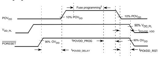
NOTE: POV<sub>DD</sub> must be stable at 1.5 V prior to initiating fuse programming.
