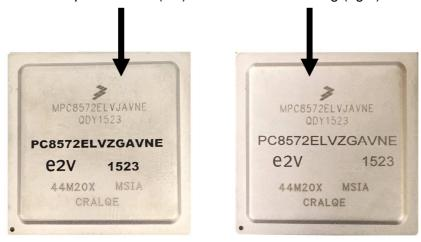
Note: The marking's characters of the component and its layout will remain unchanged.
