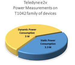
Figure 5 : T1042 power measurements at 125C
