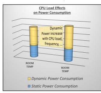
Figure 3 : Effect of CPU load on power consumption
