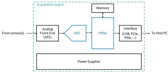
Figure 2: High-level diagram of the acquisition system
