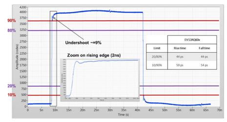
Figure 4: EV12AQ600, pulse measurement
