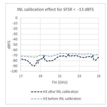
Figure 6 - Impact on H3 with INL calibration
