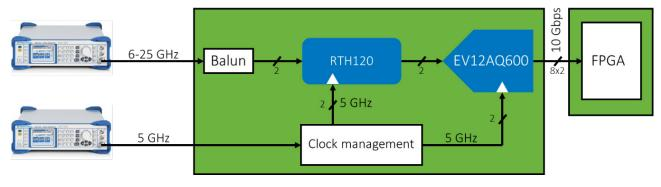
Figure 1 - FEB test evaluation set up showing key active devices
