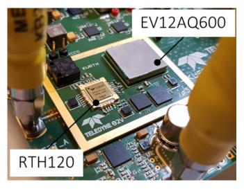
Figure 2 - Photo of initial prototype FEB on its carrier board
