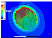
Figure 10 - Extract of a 3D field solver simulation (Ansys HFSS) of the 40GHz analog input for the PS640 showing the transition between the package and the silicon die of the THA, where signal propagation across the silicon metal filling is analyzed
