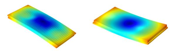
Figure 11 - 50x magnification of the PS640 packaging warpage after assembly at room temperature.
