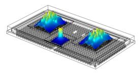
Figure 9 - Thermal Simulation of the PS640 SiP
