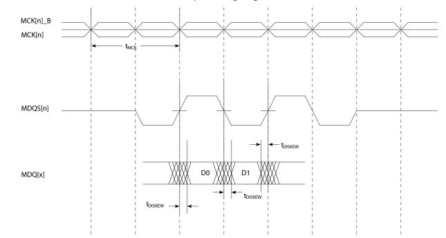
Figure 3-3. DDR3 and DDR3L SDRAM Interface Input Timing Diagram
