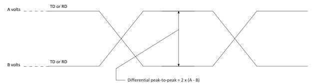
To illustrate these definitions using real values, consider the case of a CML (current mode logic) transmitter that has a common mode voltage of 2.25 V, and each of its outputs TD and TD\_B, has a swing that goes between 2.5 V and 2.0 V. Using these values, the peak-to-peak voltage swing of the signals TD and TD\_B is 500 mV p-p. The differential output signal ranges between 500 mV and –500 mV. The peak differential voltage is 500 mV. The peak-to-peak differential voltage is 1000 mV p-p.
