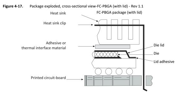
The system board designer can choose between several types of heat sinks to place on the device. There are several commercially-available thermal interfaces to choose from in the industry. Ultimately, the final selection of an appropriate heat sink depends on many factors, such as thermal performance at a given air velocity, spatial volume, mass, attachment method, assembly, and cost.
