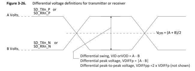
Using this waveform, the definitions are as shown in the following list. To simplify the illustration, the definitions assume that the SerDes transmitter and receiver operate in a fully symmetrical differential signaling environment:
