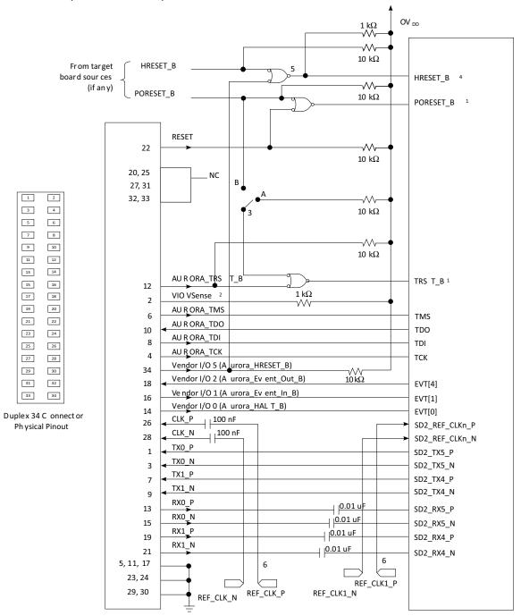
Figure 4-14. Aurora 34 pin connector duplex interface connection
