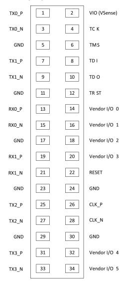
Figure 4-12. Aurora 34 pin connector duplex pinout
