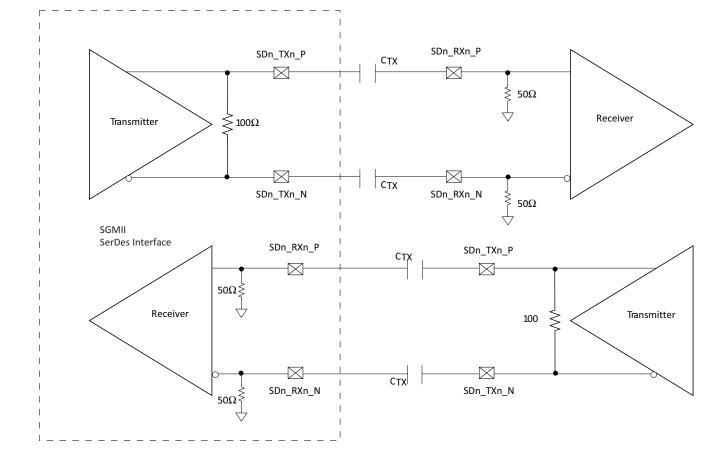
This figure shows the SGMII transmitter DC measurement circuit.
