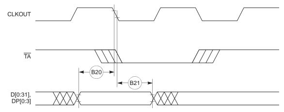
Figure 8-8. External Bus Read Timing (GPCM Controlled – ACS = '00')
