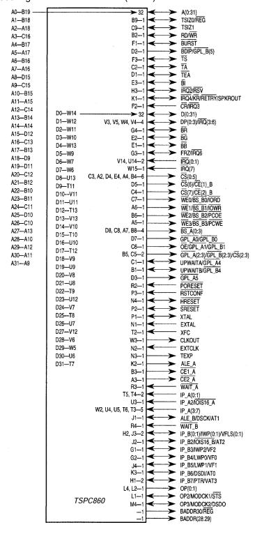
Figure 4-3. TSPC860 Signals and Pin Numbers (Part 2)
