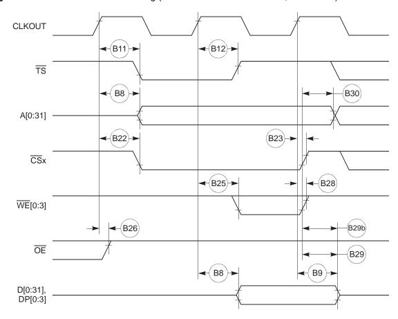
**Figure 8-12.** External Bus Write Timing (GPCM controlled – TRLX = '0', CSNT = '0')
