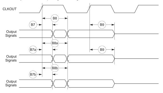
Figure 8-4. Synchronous Active Pull-up and Open Drain Output Signals Timing
