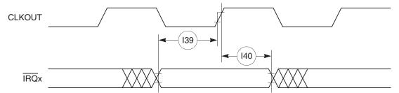
Figure 8-22. Interrupt Detection Timing for External Edge Sensitive Lines
