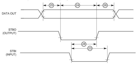
Figure 9-3. PIP RX (Pulse Mode) Timing Diagram
