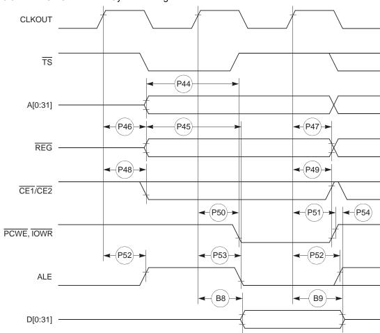
Figure 8-24. PCMCIA Access Cycles Timing External Bus Write
