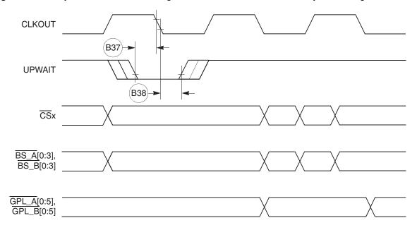
Figure 8-18. Synchronous External Master Access Timing – GPCM handled ACS = '00'
