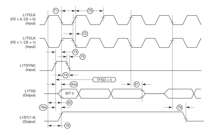
Figure 9-16. SI Transmit Timing with Double Speed Clocking (DSC = 1)
