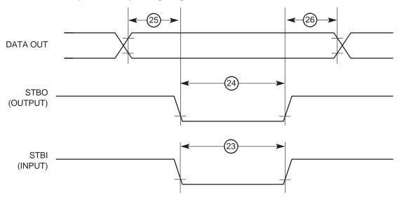
Figure 9-5. Parallel I/O Data-in/Data-out Timing Diagram
