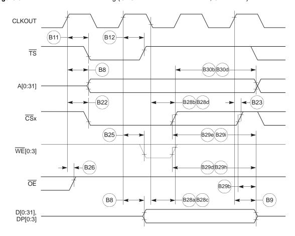
**Figure 8-14.** External Bus Write Timing (GPCM controlled – TRLX = '1', CSNT = '1')
