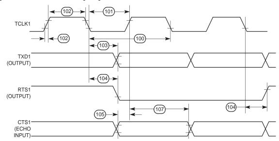
Figure 9-20. HDLC Bus Timing Diagram
