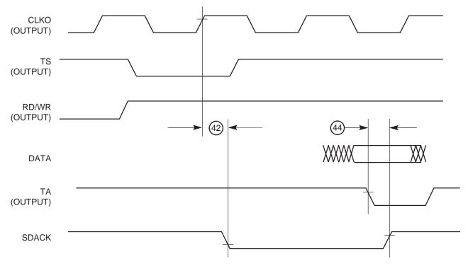
Figure 9-10. SDACK Timing Diagram – Peripheral Read
