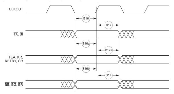
Figure 8-6. Input Data Timing in Normal Case
