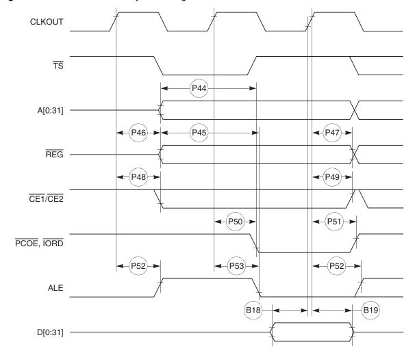
Figure 8-23. PCMCIA Access Cycles Timing External Bus Read
