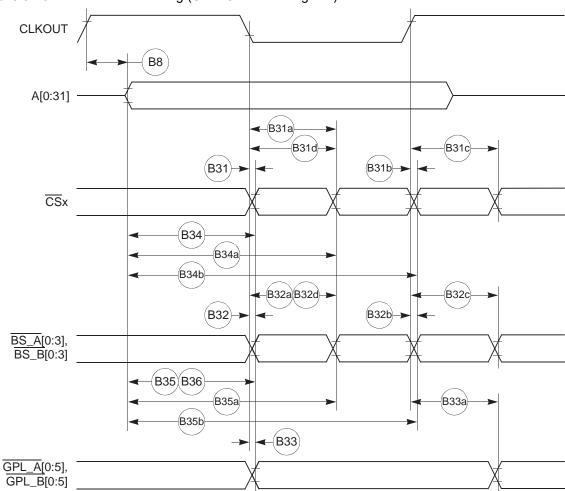
Figure 8-15. External Bus Timing (UPM Controlled Signals)
