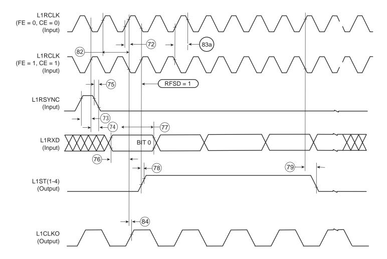
Figure 9-15. SI Transmit Timing Diagram (DSC = 0)
