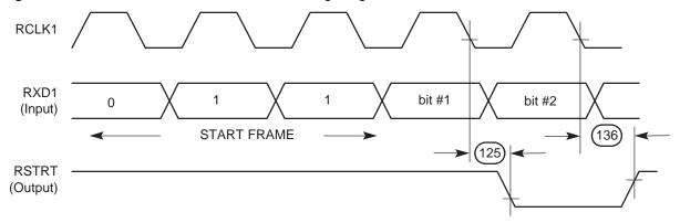
Figure 9-25. CAM Interface REJECT Timing Diagram
