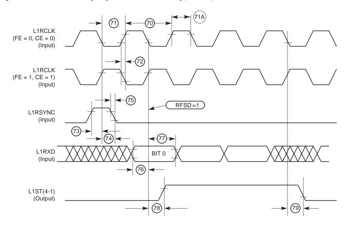
**Figure 9-14.** SI Receive Timing with Double-Speed Clocking (DSC = 1)
