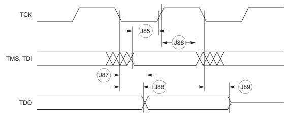
Figure 8-35. JTAG – TRST Timing Diagram
