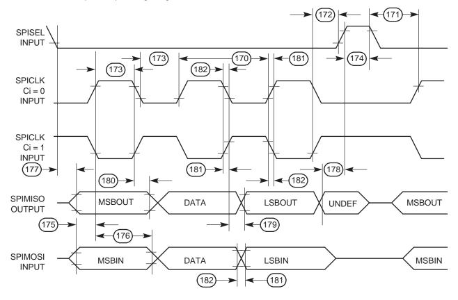
Figure 9-30. SPI Slave (CP = 1) Timing Diagram
