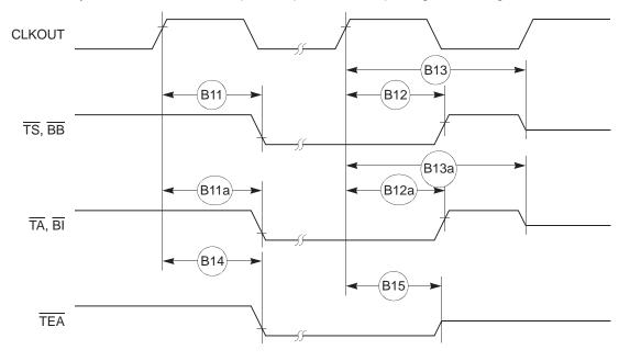
Figure 8-5. Synchronous Input Signals Timing
