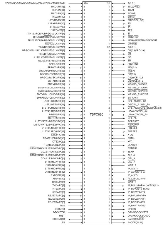
**Figure 4-2.** TSPC860 Signals and Pin Numbers (Part 1)
