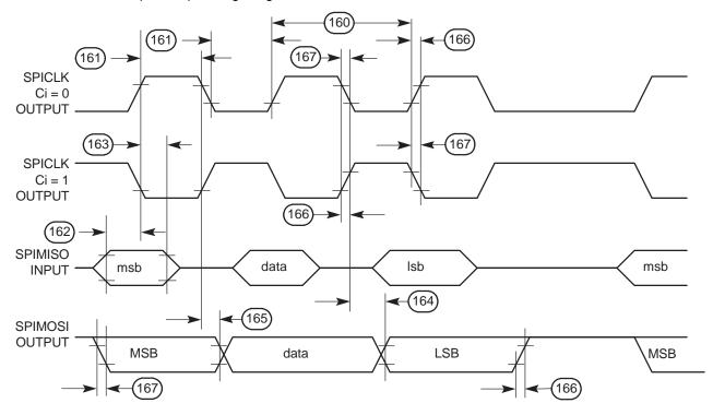
Figure 9-28. SPI Master (CP = 1) Timing Diagram
