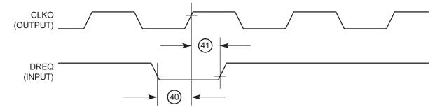
**Figure 9-8.** SDACK Timing Diagram – Peripheral Write, TA Sampled Low at the Falling Edge of the Clock
