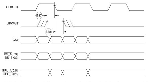
Figure 8-17. Asynchronous UPWAIT Negated Detection in UPM Handled Cycles Timing
