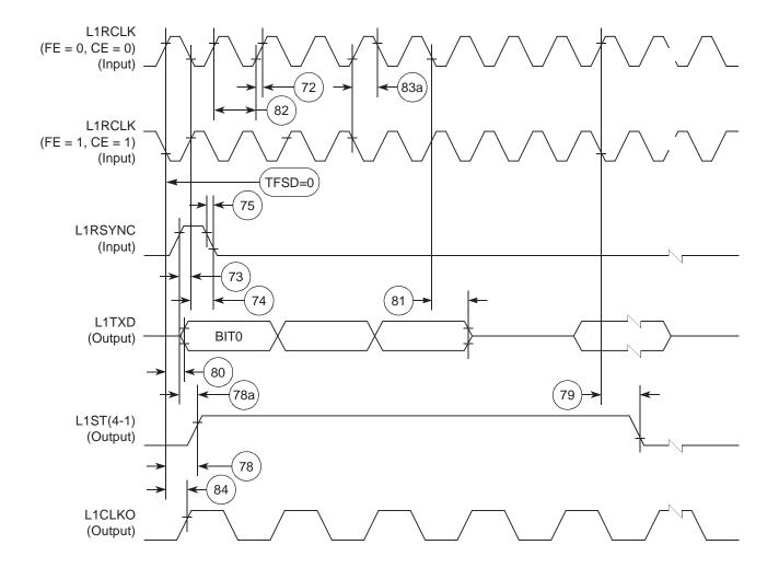
Figure 9-17. IDL Timing 1 1 2 1 3 1 4 1 5 1 6 1 7 1 8 1 3 1 1 1 1 2 1 3 1 1 4 1 1 5 1 1 8 1 3 1 3 1 3 1 4 1 5 1 6 1 7 1 8 1 3 1 3 1 3  $|B26 \times B25 \times B24 \times B23 \times B22 \times B21 \times B20 \times B20 \times B20 \times B21 \times B20 \times B20$ B25 X B24 X B23 X B22 X B21 X B20 > (B26) 8 B27 B12XB11XB10XD1 (B16 \ B15 \ B14 \ B13 \ 87 B15 \ B14 \ \ B16 85 86
