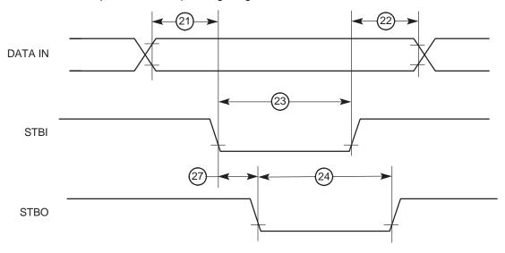
Figure 9-2. PIP TX (Interlock Mode) Timing Diagram
