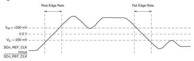
Figure 3-38. Single-Ended Measurement Points for Rise and Fall Time Matching
