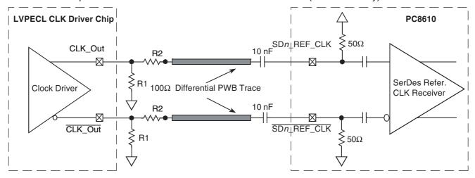
Figure 3-36 shows the SerDes reference clock connection reference circuits for a single-ended clock driver. It assumes the DC levels of the clock driver are compatible with PC8610 SerDes reference clock input's DC requirement.
