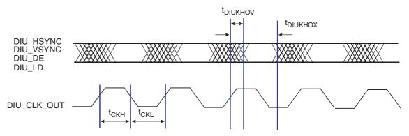
Note: The DIU\_OUT\_CLK edge and phase delay is selectable via the Global Utilities CKDVDR register.
