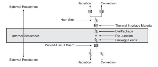
Note the internal versus external package resistance
