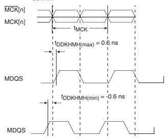
Figure 3-5 shows the DDR SDRAM output timing diagram.
