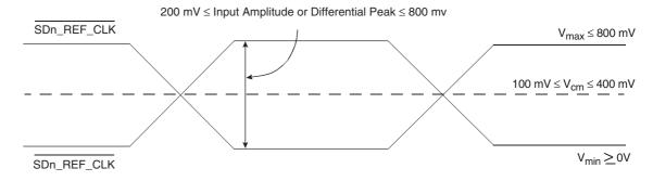
Figure 3-31. Differential Reference Clock Input DC Requirements (External AC-Coupled)
