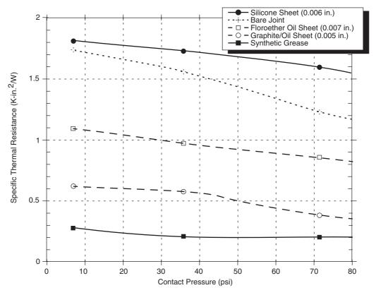
The board designer can choose between several types of thermal interface. Heat sink adhesive materials should be selected based on high conductivity and mechanical strength to meet equipment shock/vibration requirements. There are several commercially available thermal interfaces and adhesive materials provided by the following vendors:
