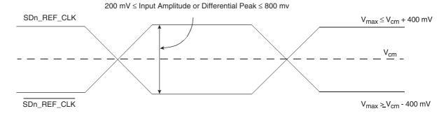
Figure 3-32. Single-Ended Reference Clock Input DC Requirements
