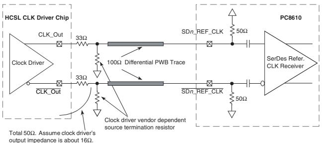
Figure 3-34 shows the SerDes reference clock connection reference circuits for LVDS type clock driver. Since LVDS clock driver's common mode voltage is higher than the PC8610 SerDes reference clock input's allowed range (100 to 400 mV), AC-coupled connection scheme must be used. It assumes the LVDS output driver features  $50\Omega$  termination resistor. It also assumes that the LVDS transmitter establishes its own common mode level without relying on the receiver or other external component.
