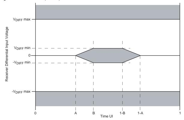
Figure 17-3. Receiver Input Compliance Mask
