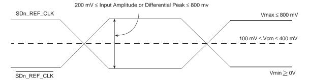
Figure 15-4. Differential Reference Clock Input DC Requirements (External AC-Coupled)
