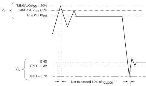
**Figure 2-1.** Overshoot/Undershoot Voltage for TV<sub>DD</sub>/BV<sub>DD</sub>/GV<sub>DD</sub>/LV<sub>DD</sub>/OV<sub>DD</sub>
