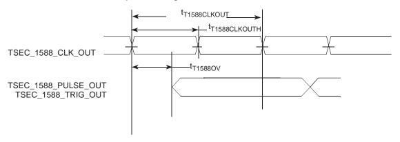
Note: 1. The output delay is count starting rising edge if t<sub>T1588CLKOUT</sub> is non-inverting. Otherwise, it is count starting falling edge.
