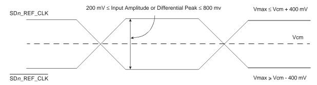
Figure 15-5. Single-Ended Reference Clock Input DC Requirements
