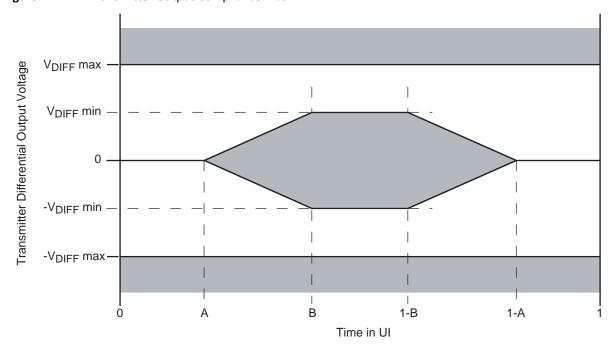
Figure 17-1. Transmitter Output Compliance Mask
