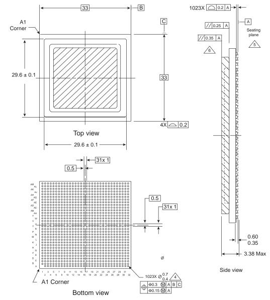
Figure 18-1. Mechanical Dimensions of the PC8572E FC-PBGA with Full Lid
