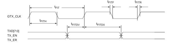
Figure 8-2. FIFO Receive AC Timing Diagram
