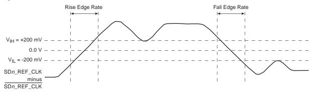
Figure 15-11. Single-Ended Measurement Points for Rise and Fall Time Matching
