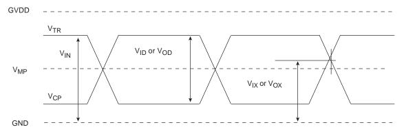
Note: VID specifies the input differential voltage |VTR -VCP| required for switching, where VTR is the <a href="true">true</a> input signal (such as MCK or MDQS) and VCP is the complementary input signal (such as MCK or MDQS).
