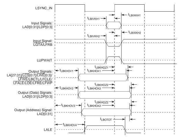
Table 10-7 describes the general timing parameters of the local bus interface at  $BV_{DD} = 3.3V$  DC with PLL disabled.
