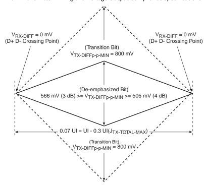
Figure 16-1. Minimum Transmitter Timing and Voltage Output Compliance Specifications
