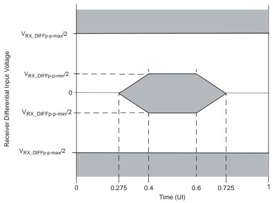
Figure 8-19. SGMII AC Test/Measurement Load
