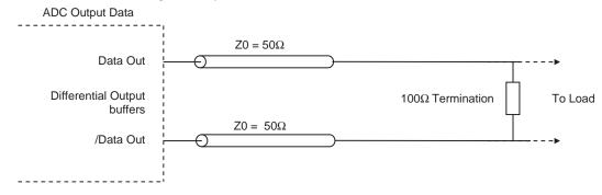
If the ADC is used in 1:1 or 1:2 DMUX modes, the unused ports can be left open (no external termination required).
