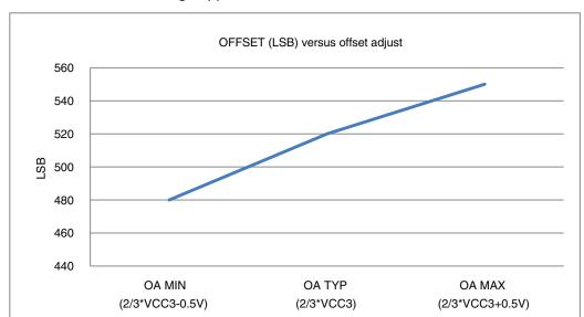
Figure 5-2. Offset Versus Voltage Applied on OA
