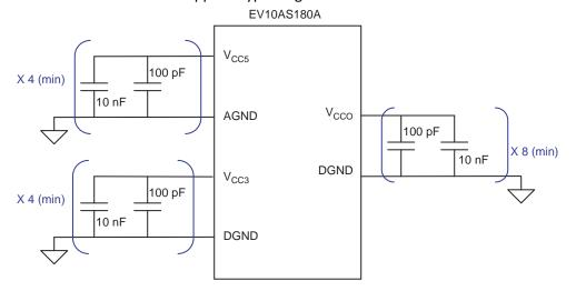
Each power supply has to be bypassed as close as possible to its source or access by 100 nF in parallel to  $1 \mu F$  capacitors.
