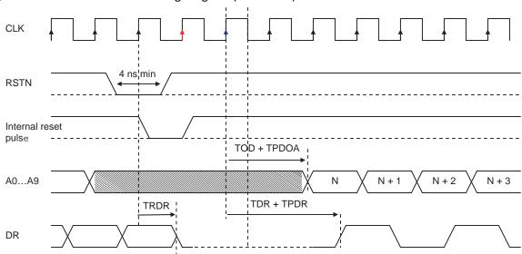
Figure 2-5. External Reset Timing Diagram (1:1 DMUX)
