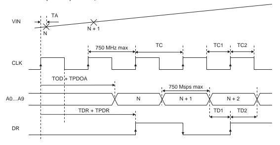
Figure 2-2. Principle of Operation, DMUX 1:2
