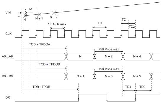
Figure 2-3. Principle of Operation, DMUX 1:4
