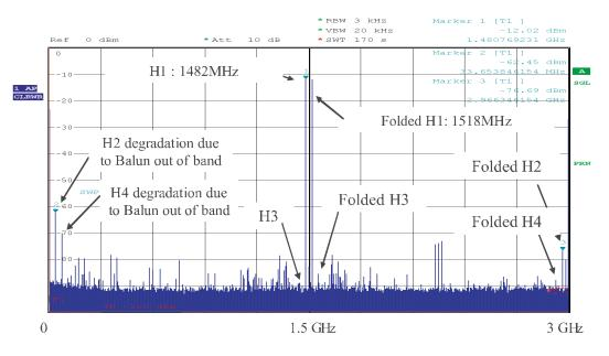
On the opposite, when appropriate balun is used the real device response is measured.
