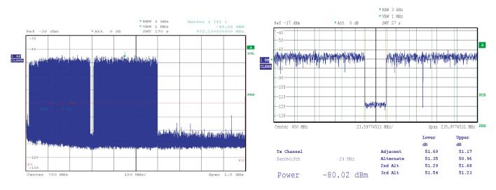
Measured average NPR: 51.36 dB, therefore SNR = 62.36 dB and ENOB = 10.07 bit.
