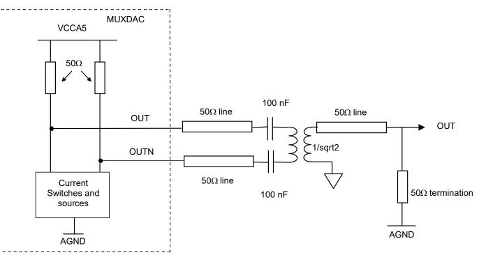
Note: The AC coupling capacitors should be chosen as broadband capacitors with a value depending on the application.
