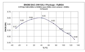
Optimum is at Tj = 40°C, degradation over temp is within 1 dB (or 0.15 effective bit).
