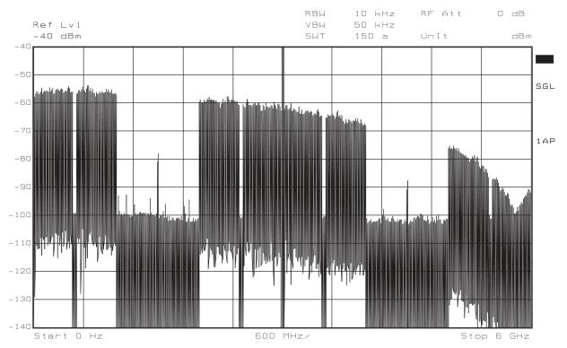
First Zero of the sinc() function is slightly before 2\*Fclock which indicates that the duty cycle of RTZ function is a little bit more than 50%, this is due to the balun which introduced some phase error beyond the 180 degrees between CLK and CLKN thus creating a duty cycle on the clock actually seen by the DAC.
