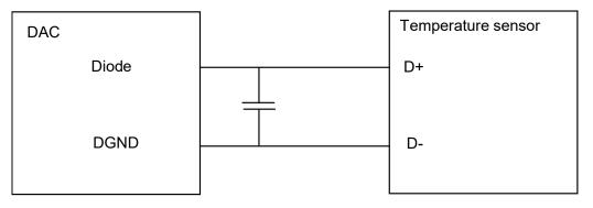
In characterization measurement a current of 1 mA is applied on the DIODE pin. The voltage across the DIODE pin and the DGND pin gives the junction temperature using the intrinsic diode characteristics below Figure 5-19.
