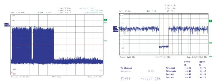
Measured average NPR: 44.6 dB, therefore SNR = 55.6 dB and ENOB = 8.94 bit
