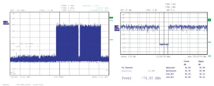
Measured average NPR: 42.56 dB, therefore SNR = 53.56 dB and ENOB = 8.6 bit.
