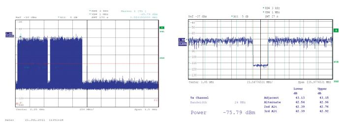
Measured average NPR: 42.78 dB, therefore SNR = 53.78 dB and ENOB = 8.64 bit
