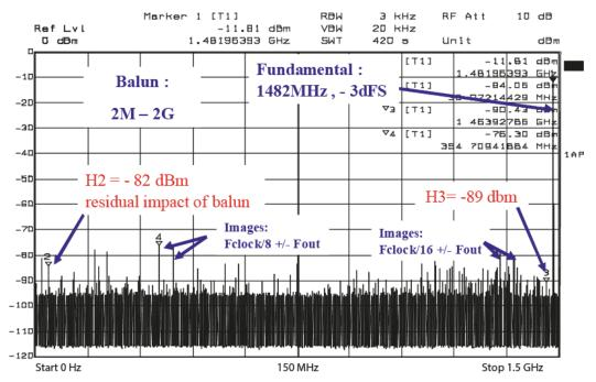
As a consequence, one must be aware that optimum performances can only be reached when using a balun optimal for the band of interest of the application. We specifically recommend selecting a balun which frequency domain covers the whole band of interest (for instance one whole Nyquist zone).
