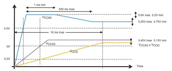
The rise time for any of the power supplies (V<sub>CCA5</sub>, V<sub>CCA3</sub> and V<sub>CCD</sub>) shall be  $\leq$  10 ms.
