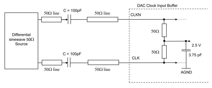
Note: The buffer is internally pre-polarized to 2.5V (buffer between V<sub>CC5</sub> and AGND).
