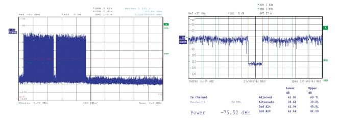
Measured average NPR: 40.08 dB, therefore SNR = 51.08 dB and ENOB = 8.19 bit
