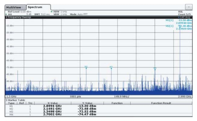
Figure 7-24. Typical SFDR spectrum in RF mode. Fout = 4400MHz (3rd Nyquist), MUX4:1, Fs = 3Gsps. SFDR = 56 dBc
