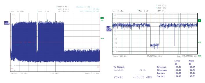
Measured average NPR: 50.02 dB, therefore SNR = 61.02 dB and ENOB = 9.84 bit Effects at low frequency are due to balun and pattern.
