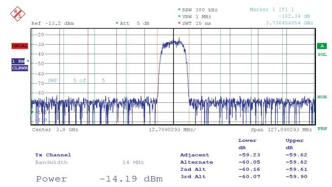
Figure 7-31. RF Mode, 3rd Nyquist Zone: Center Frequency is pushed to 3 GHz+ 800 MHz = 3.8 GHz
