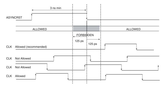
**Figure 4-1.** CLK to ASYNCRST Timing with V(CLKDACTRL) = 1.1V
