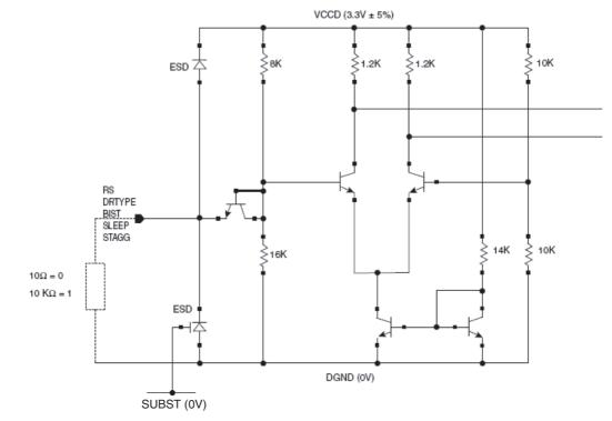
Figure 8-4. Control Signals Input Buffers: BIST, STAGG, SLEEP, RS, DRTYPE
