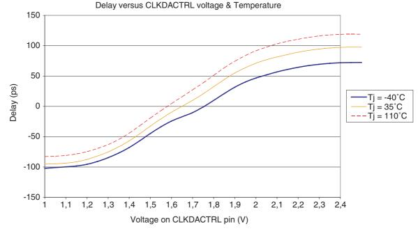
The tuning range is varying linearly over the specified temperature range. The longest tuning range is obtained at hot temperature.
