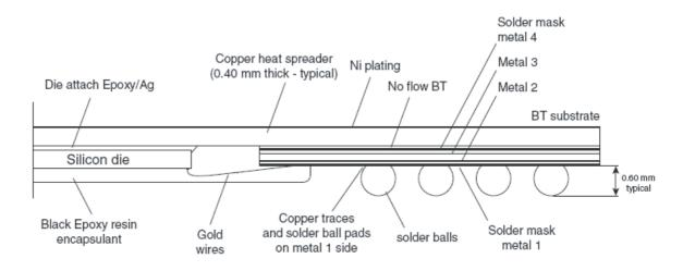
Note: In the DMUX package (see above), the die's underside is attached to the copper heat spreader so the copper heat spreader is at GND (0V).
