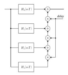
Where :  $\begin{aligned} &H_0(\omega T)\approx 1\\ &H_1(\omega T)\approx -j\omega T\\ &H_2(\omega T)\approx -(\omega T)^2/2\\ &H_3(\omega T)\approx j(\omega T)^3/6 \end{aligned}$
