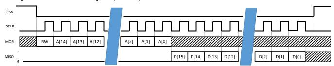
Figure 16 - SPI reading timing
