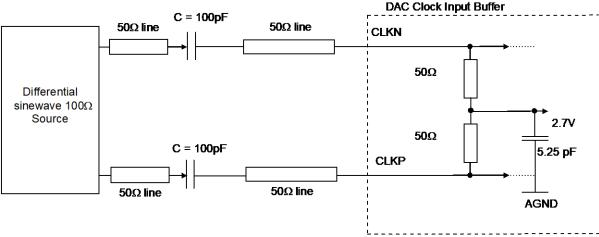
Figure 67: Clock input differential with balun
