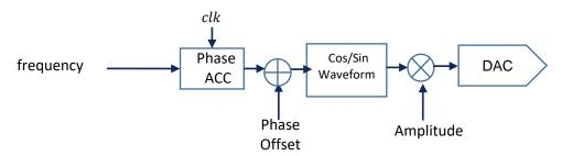
Figure 42 - Direct Digital Synthesis Principle
