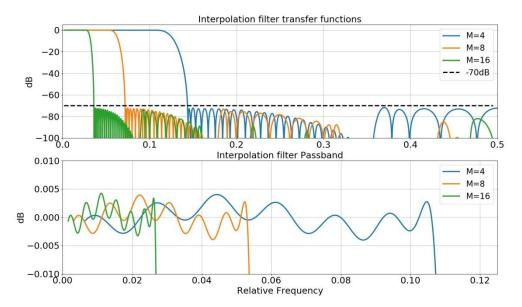
Figure 35 - Interpolation filter for orders 4, 8 and 16 and bandpass behavior for each order.
