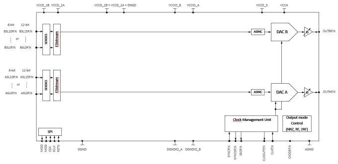
Figure 2: Simplified Block Diagram using Real data
