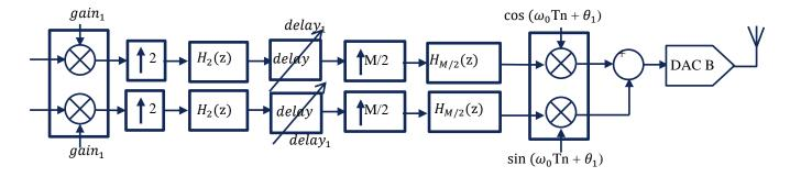
Figure 40 - Beam-forming (Digital Butler Matrix) principle
