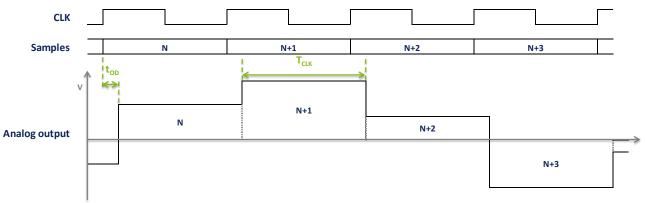
Figure 28 - NRZ mode timing diagram
