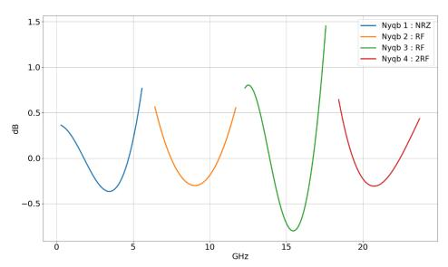
Figure 58 - Remaining error after anti-sinc compensation (Fs = 12 GSps)
