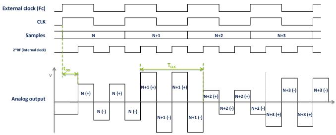
Figure 30 - 2RF mode timing diagram
