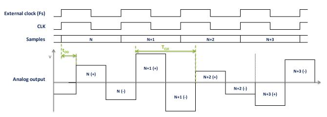
Figure 29 - RF mode timing diagram
