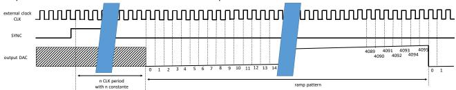
Figure 59: Ramp test mode timing diagram
