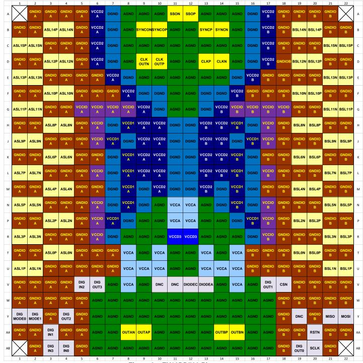
Figure 8 – EV12DD700 Pinout
