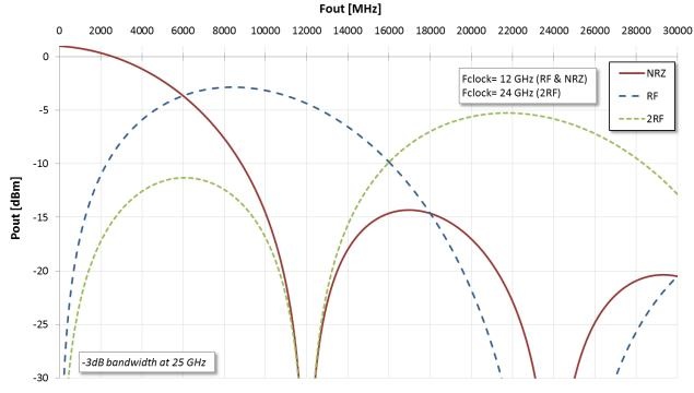
Figure 3: Output DAC response at 12GSps in NRZ and RF mode and 2RF mode with 24GHz clock (include the attenuation due to 25GHz output bandwidth, but does not include additional attenuation due to internal parasitics)
