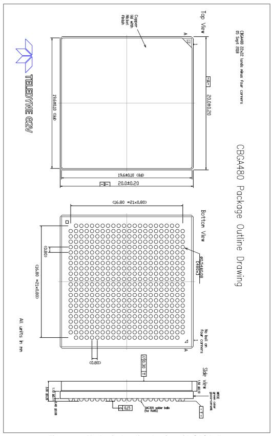
Figure 13 - Mechanical outline drawing with SAC balls
