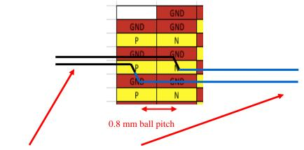
Length on board and length on package are almost the same on N and P (less routing on board for P results from more routing inside package for P).
