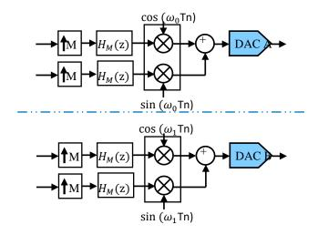
Figure 38 - Digital Up Conversion Block diagram
