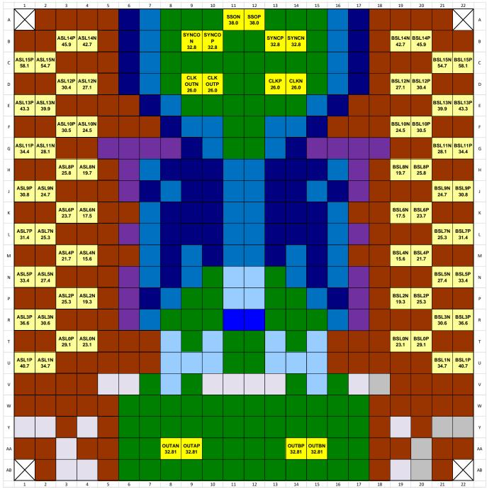
Figure 10 - EV12DD700 relative skews on HSSL, AOUT and Clock signals (values are in ps)
