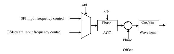
Figure 49 - Frequency Hopping Principle
