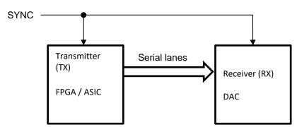
Figure 22: SYNC pulse sequence principle between ESIstream transmitter and receiver
