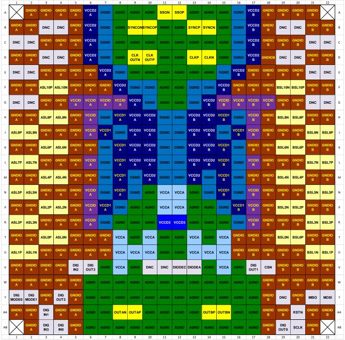
Figure 7 - EV8DD700 Pinout
