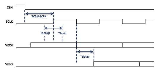
Figure 6 - SPI timing diagram
