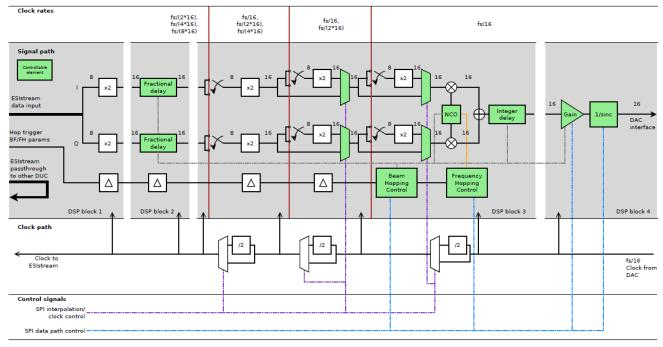
Figure 32 - Signal path with DUC
