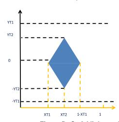
Figure 5 - Serial link eye diagram
