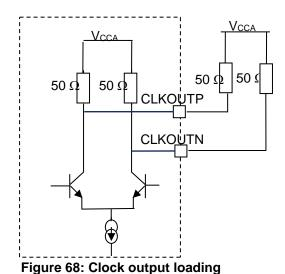
If not used CLKout output buffer can be turned OFF and can remain open.
