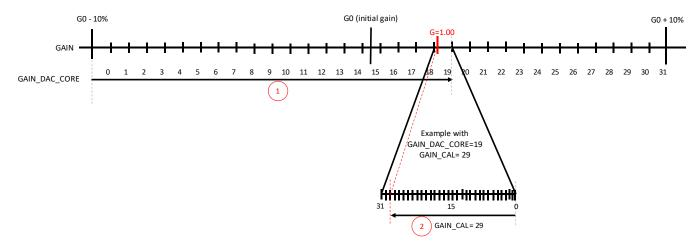
Figure 26: Gain adjustment trough x\_GAIN\_CAL & GAIN\_DAC\_CORE
