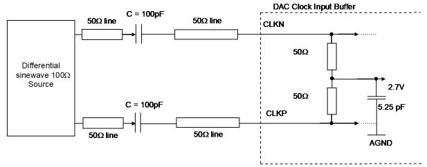
Figure 66: Clock input differential termination
