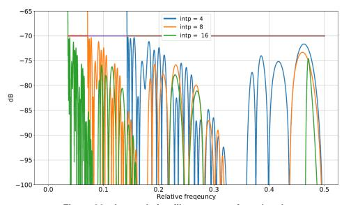
Figure 36 - Interpolation filters, zoom of stopband
