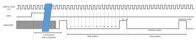
Figure 61: Flash test mode timing diagram (double size maximum value)
