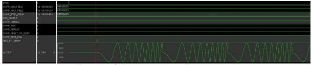
Figure 48 - Chirp mode - Automatic repeat pattern
