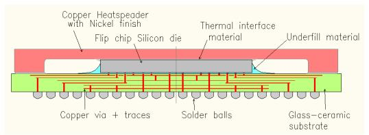
Figure 12 - Ceramic package cross-section
