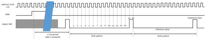
Figure 60: Flash test mode timing diagram
