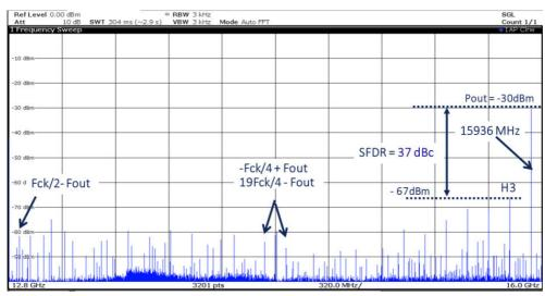
Figure 57. Typical SFDR spectrum in RF mode with Fout = 19146 MHz ( $6^{th}$  Nyquist), MUX4:1, Fs = 6.4 GSps, SFDR = 43 dBc
