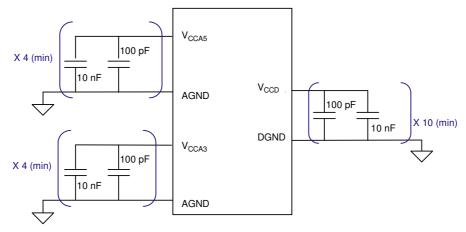
Each power supply has to be bypassed as close as possible to its source and accessed by 100 nF in  $\,$  parallel to 22  $\,$   $\mu$ F capacitors (the optimum value depends on the regulators).
