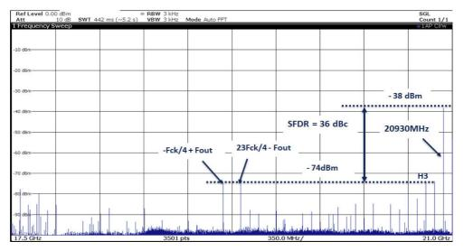
Figure 66. Typical SFDR spectrum in RF mode with Fout = 24430 MHz ( $7^{th}$  Nyquist), MUX4:1, Fs = 7.0 GSps, SFDR = 37 dBc
