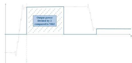
Figure 16. DAC output in RTZ mode and time domain when RPB is optimum
