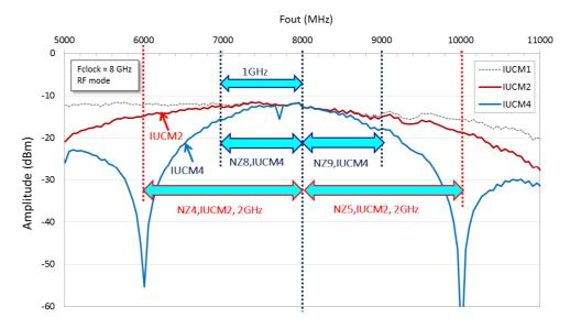
Figure 47. Pout vs Fout @ 8.5 GSps from DC to 26 GHz, IUCM1, IUCM2 and IUCM4 in RF mode
