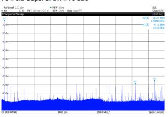
Figure 77.Typical SFDR spectrum in NRTZ mode. Fout = 1568 MHz (1<sup>st</sup> Nyquist), MUX2:1, Fs = 3.2 GSps. SFDR = 65 dBc
