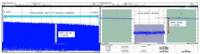
Measured average NPR: 38 dB, therefore SNR = 49 dB and ENOB = 7,85 bit
