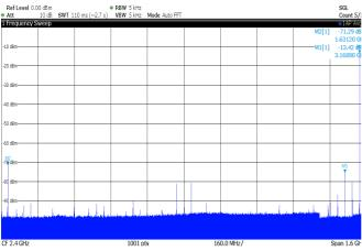
Figure 76. Typical SFDR spectrum in NRTZ mode. Fout = 32 MHz (1<sup>st</sup> Nyquist), MUX2:1, Fs = 3.2 GSps. SFDR = 76 dBc
