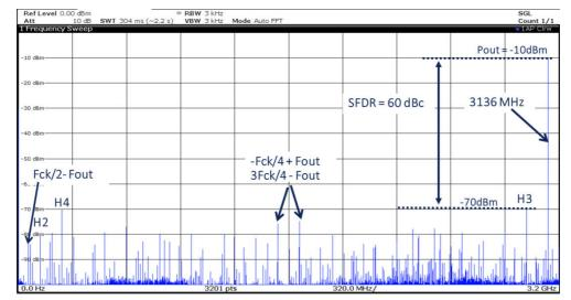
Figure 53. Typical SFDR spectrum in NRTZ mode with Fout = 6336 MHz ( $2^{nd}$  Nyquist), MUX4:1, Fs = 6.4 GSps, SFDR = 53 dBc
