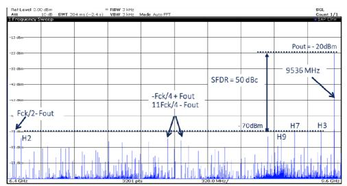
Figure 55. Typical SFDR spectrum in RF mode with Fout = 12736 MHz ( $4^{th}$  Nyquist), MUX4:1, Fs = 6.4 GSps, SFDR = 48 dBc
