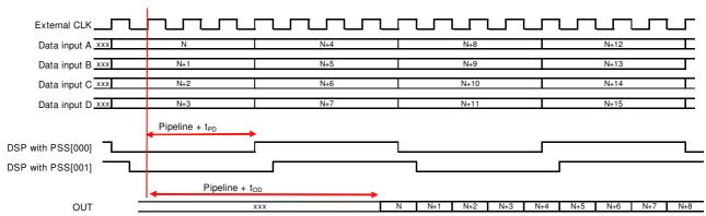
Figure 3. Timing diagram for 4:1 MUX principle of operation, IUCM2
