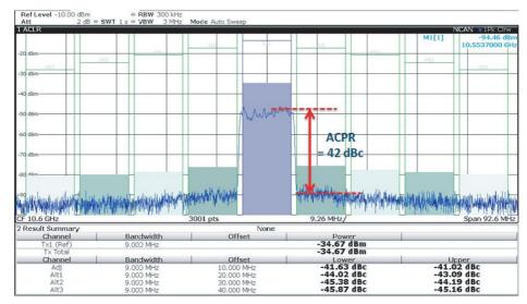
Figure 97. Adjacent Channel Power Ratio (ACPR) @ 6.0 GSps, 10 MHz QPSK, 16.6 GHz Center frequency, ACPR = 36.7 dBc, RF mode
