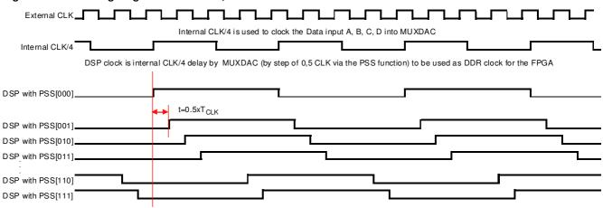
Figure 23. PSS timing diagram for 2:1 MUX, OCDS = 0
