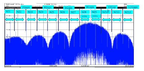
Figure 113. NPR vs Output Frequency at 8.0 Gsps in IUCM2 in RF mode in NZ4 (4<sup>th</sup> Nyquist zone)
