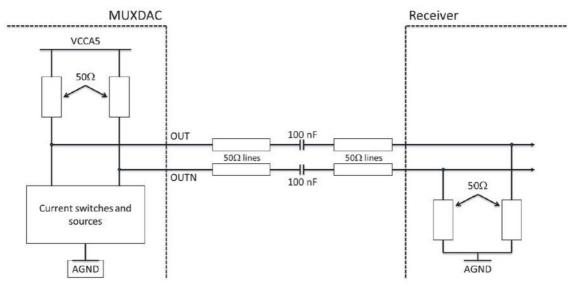
Figure 124. Analog output using a 1/sqrt(2) Balun
