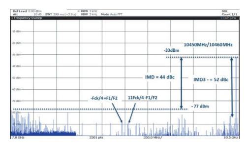
Figure 93. Typical Dual-tone spectrum in NRTZ mode with Fout1,Fout2 = 13950 MHz,13960 MHz, (4<sup>th</sup> Nyquist), MUX4:1, Fs = 7.0 GSps, IMD3 - = 54 dBc, IMD full Nyquist = 48 dBc
