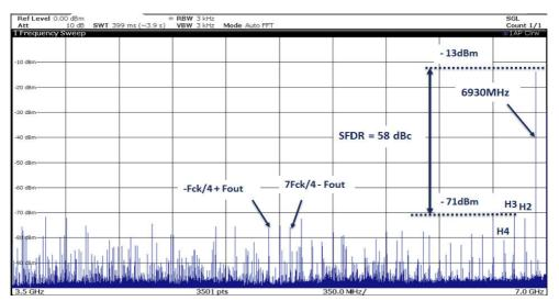
Figure 62. Typical SFDR spectrum in RF mode with Fout = 10430 MHz ( $3^{rd}$  Nyquist), MUX4:1, Fs = 7.0 GSps, SFDR = 50 dBc
