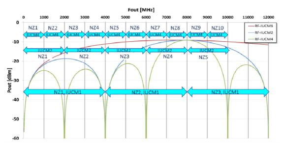
Figure 26. Pout curves in RF mode at 8.0 GSps from DC to 12 GHz in IUCM1, IUCM2 and IUCM4 modes
