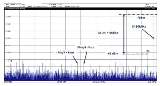
Figure 61. Typical SFDR spectrum in RF mode with Fout = 6930 MHz ( $2^{\text{nd}}$  Nyquist), MUX4:1, Fs = 7.0 GSps, SFDR = 58 dBc
