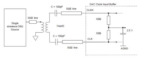
The AC coupling capacitors should be chosen as broadband capacitors with a value depending on the application).
