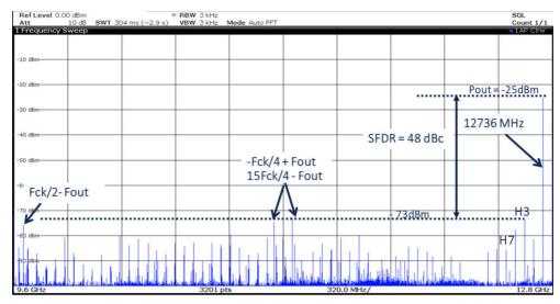
Figure 56. Typical SFDR spectrum in NRTZ mode with Fout = 15936 MHz ( $5^{th}$  Nyquist), MUX4:1, Fs = 6.4 GSps, SFDR = 37 dBc
