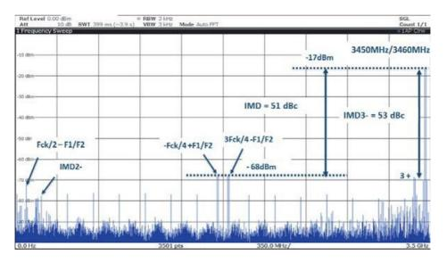
Figure 91. Typical Dual-tone spectrum in RF mode with Fout1,Fout2 = 6950 MHz,6960 MHz (2<sup>nd</sup> Nyquist), MUX4:1, Fs = 7.0 GSps, IMD3 - = 64 dBc, IMD full Nyquist = 59 dBc
