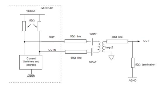
Note: The AC coupling capacitors should be chosen as broadband capacitors with a value depending on the application.
