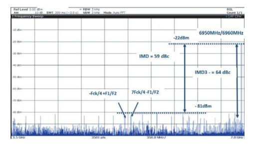
Figure 92. Typical Dual-tone spectrum in RF mode with Fout1,Fout2 = 10450 MHz,10460 MHz (3<sup>rd</sup> Nyquist), MUX4:1, Fs = 7.0 GSps, IMD3 - = 52 dBc, IMD full Nyquist = 44 dBc
