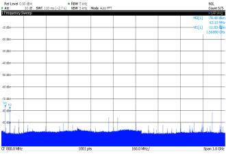
Figure 79. Typical SFDR spectrum in RF mode. Fout = 3168 MHz (2<sup>nd</sup> Nyquist), MUX2:1, Fs = 3.2 GSps. SFDR = 58 dBc
