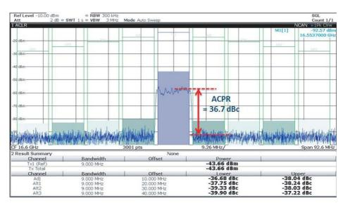
Figure 98. Adjacent Channel Power Ratio (ACPR) @ 6.0 GSps, 10 MHz QPSK, 22.6 GHz Center frequency, ACPR = 30 dBc, RF mode
