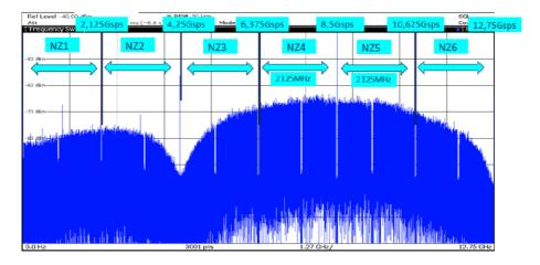
Figure 118. NPR vs Output Frequency at 8.5 Gsps in IUCM4 in RF mode over 6 Nyquist zones
