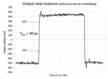
After the oscilloscope probe de-embedding,  $T_{rise} \approx 30 \text{ ps} \rightarrow DAC \text{ bandwidth} \approx 7.5 \text{ GHz}$
