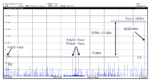
Figure 54. Typical SFDR spectrum in RF mode with Fout = 9536 MHz ( $3^{rd}$  Nyquist), MUX4:1, Fs = 6.4 GSps, SFDR = 50 dBc
