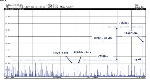
Figure 64. Typical SFDR spectrum in RF mode with Fout = 17430 MHz ( $5^{th}$  Nyquist), MUX4:1, Fs = 7.0 GSps, SFDR = 41 dBc
