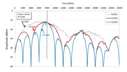
Figure 46. Pout vs Fout @ 8.0 GSps from 5GHz to 11 GHz, IUCM1, IUCM2 and IUCM4 in RF mode
