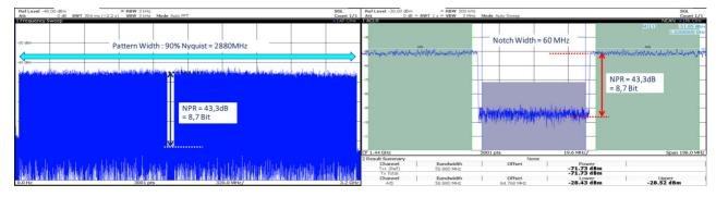
Measured average NPR: 43.5 dB, therefore SNR = 54,3 dB and ENOB = 8.7 bit
