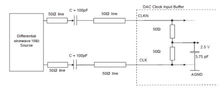
Note: The buffer is internally pre-polarized to 2.5V (buffer between  $V_{CCA5}$  and AGND).
