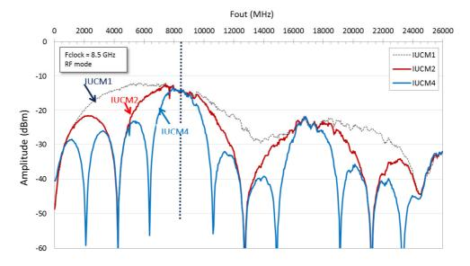
Figure 48. Pout vs Fout @ 8.5 GSps from 5.3125 GHz to 11.6875 GHz , IUCM1, IUCM2 and IUCM4 in RF mode
