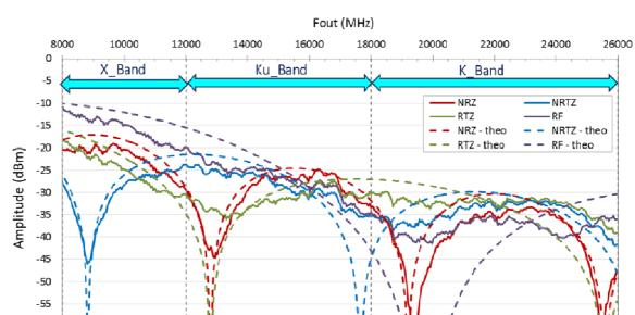
Figure 41. Pout vs Fout @ 6.4 GSps from 8 GHz to 26 GHz vs modes (includes X-Band, Ku-Band and K Band)
