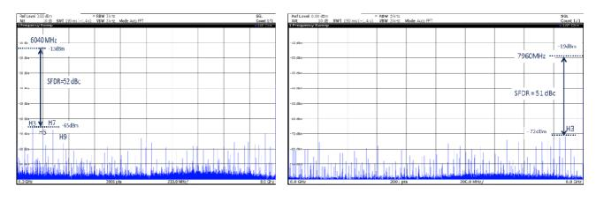
Figure 68. Typical SFDR spectrum in RF mode in IUCM2 Mode in NZ5 (Fout = 8040 MHz) and Fout = 9960 MHz, Fs = 8.0 GSps
