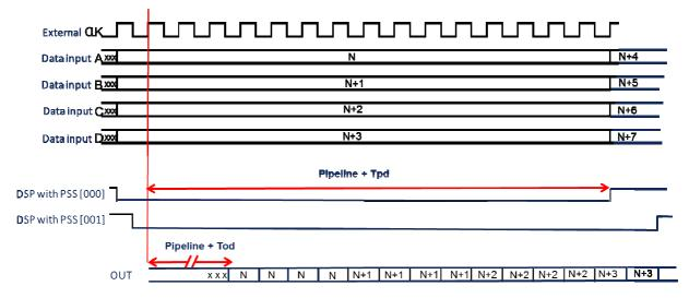
Figure 5. Timing Diagram for 2:1 MUX principle of operation OCDS1, IUCM1
