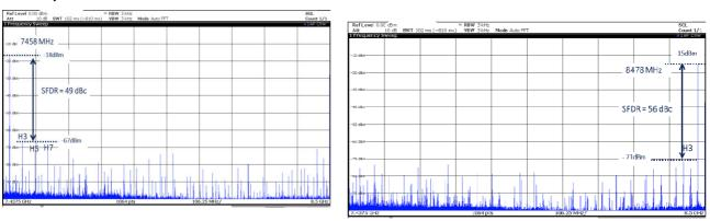
Figure 74. Typical SFDR spectrum in RF mode in IUCM4 Mode in NZ9 (Fout = 8521 MHz) and (Fout = 9541 MHz), Fs = 8.5 GSps
