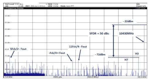
Figure 63. Typical SFDR spectrum in RF mode with Fout = 13930 MHz ( $4^{th}$  Nyquist), MUX4:1, Fs = 7.0 GSps, SFDR = 48 dBc
