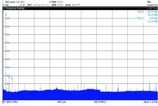
Figure 78. Typical SFDR spectrum in RTZ mode. Fout = 3168 MHz (2<sup>nd</sup> Nyquist), MUX2:1, Fs = 3.2 GSps. SFDR = 59 dBc
