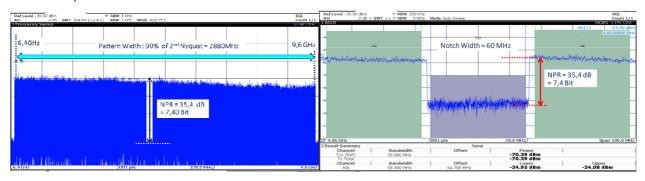
Measured average NPR: 35,4 dB, therefore SNR = 46,4 dB and ENOB = 7.4 bit
