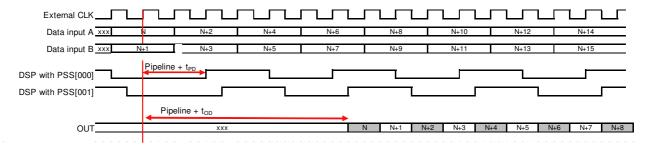
Figure 6. Timing relationship between SYNC and DSP
