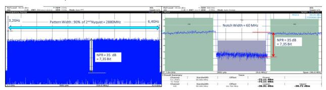
Measured average NPR: 35 dB, therefore SNR = 46 dB and ENOB = 7.35 bit
