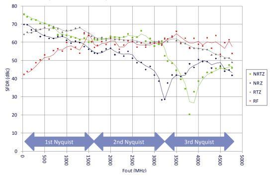
Figure 51. SFDR (dBc) vs Fout from 5 GHz to 35 GHz (covering X-Band, Ku-Band, K-Band and Ka-Band) @ 6.4 GSps in MUX4:1, RF mode
