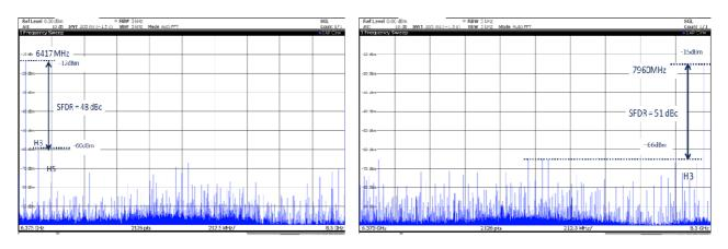
Figure 72. Typical SFDR spectrum in RF mode in IUCM2 Mode in NZ5 (Fout = 8542 MHz) and (Fout = 10582 MHz), Fs = 8.5 GSps
