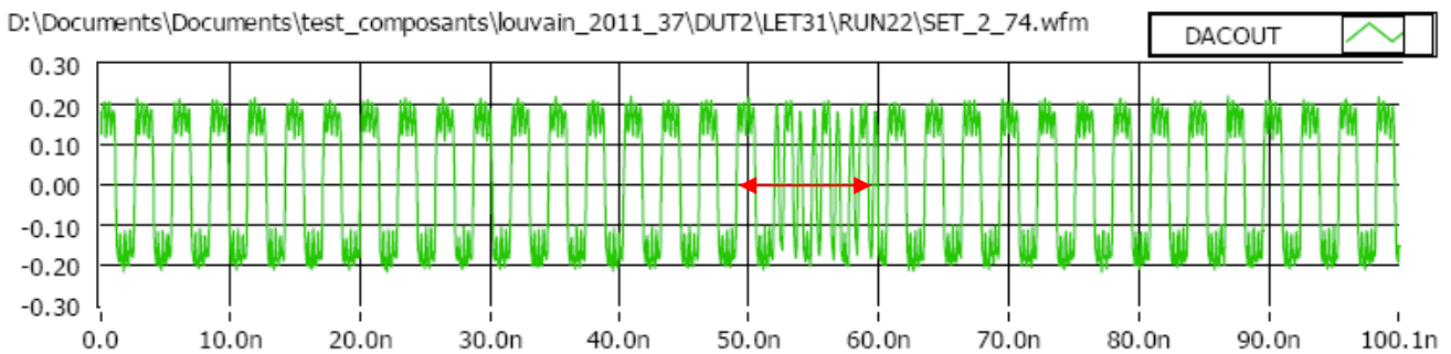
Figure 13 – Example of temporary mode change on DACOUT at 2760MHz, in NRTZ mode, LET = 31 MeV.cm 2 /mg
