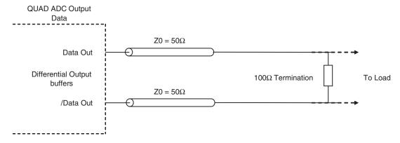
Note: If not used, leave the pins of the differential pair open
