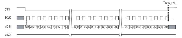
Note: Last falling edge of sclk should occur only once csn is back to high level at the end of the write procedure.
