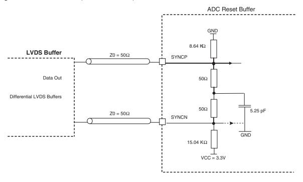
Note: If not used, leave the pins of the differential pair open
