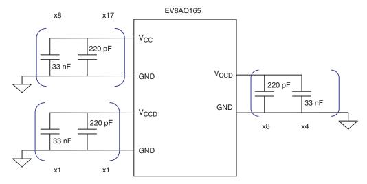
Each power supply has to be bypassed as close as possible to its source or access by 100 nF in parallel to 1 µF capacitors.
