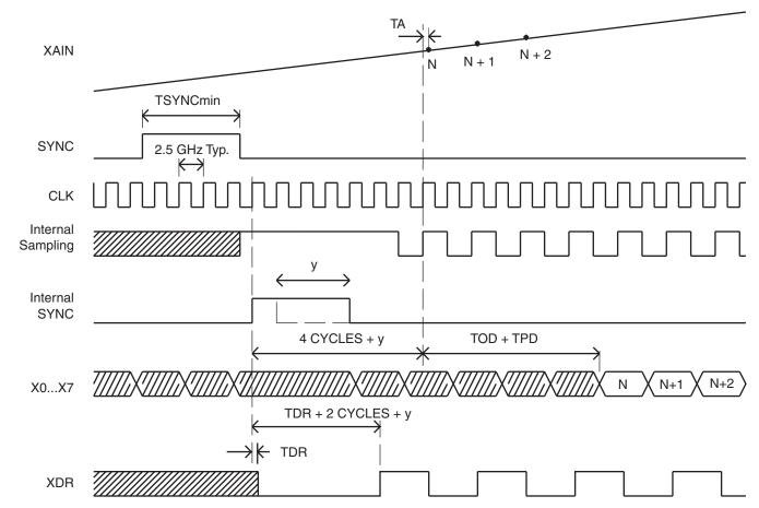
Figure 6-3. ADC SYNC Timing Condition
