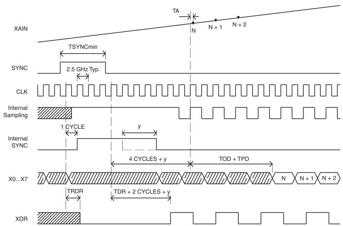
Figure 6-1. ADC SYNC Timing in Four-channel Mode, RM = 0, SYNC Register y = 3 (Tunable 0 to 15 Cycles
