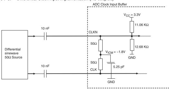
Differential mode is the recommended input scheme.
