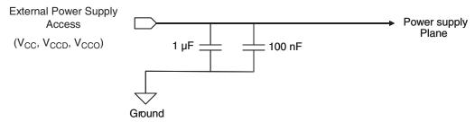
Note:  $V_{CCD}$  and  $V_{CCO}$  planes should be separated but the two power supplies can be reunited by a strap on the board.
