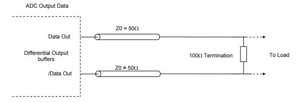
Each Digital output should always be terminated by  $100\Omega$  differential resistor placed as close as possible to differential receiver.
