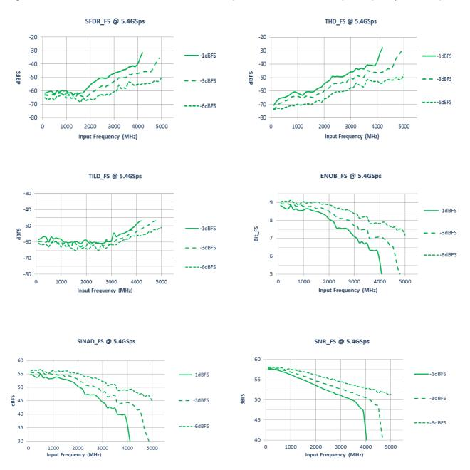
Typical supplies - at ambient temperature - 4 cores interleaved (Staggered mode).
