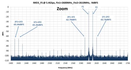
Figure 47. IMD3 at 5.4GSps Fin1 = 2600MHz, Fin2 = 2610 MHz, -12dBFS
