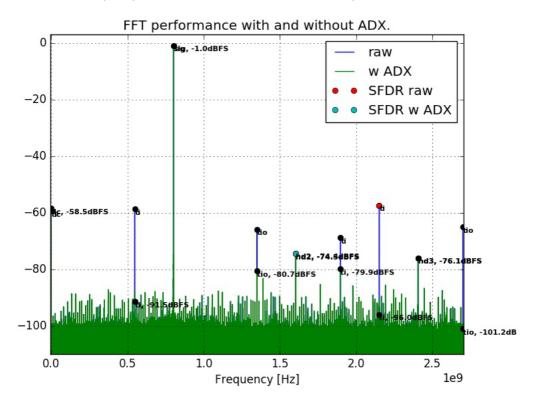
Figure 50. TI-spur height with and without ADX4 vs input signal frequency at 5.4Gsps
