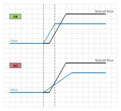
The device always starts properly when  $V_{\text{CCO}}$  is switched on first and is never overrun by the 2 other power supplies before its establishment. Once  $V_{\text{CCO}}$  has reached its steady state value, there is no constraint on  $V_{\text{CCA}}$  and  $V_{\text{CCD}}$  power-up.
