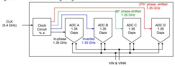
Notes: 1. For simplification purpose of the timer circuit, the temporary order of ports for sampling is A C B D, therefore sampling order at output port is as follows:
