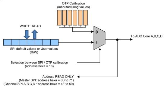
Note that reading at the READ ONLY address enables to verify the value really taken into consideration. Reading at the Read/Write address send the SPI default values or User values even if OTP calibration values are selected via OTP\_SPI\_SEL register.
