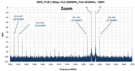
Figure 46. IMD3 at 5.4GSps Fin1 = 2600MHz, Fin2 = 2610 MHz, -9dBFS
