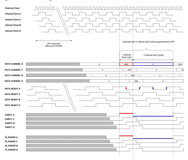
Example with FLASH\_LENGTH = 3 1 internal clock cycle = 4 external clock cycles
