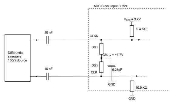
Differential mode is the recommended input scheme. Single ended input is not allowed due to performance limitations.
