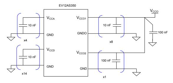
The 100nF capacitor on  $V_{CCO}$  supply between  $V_{CCO1}$  and  $V_{CCO2}$  is intended to avoid any coupling of  $V_{CCO1}$  noise (output buffers) on  $V_{CCO2}$  (digital supply) and reciprocally.
