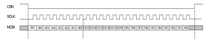
D[15] is the MSB of the 16 bit data word D[0] is the LSB of the 16 bit data word A[6] is the MSB of the 7 bit address word A[0] is the LSB of the 7 bit address word Bit RW = 1 for writing
