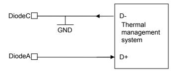
Note: If the diode function is not used, the diode pins can be left unconnected (open). If diode is used it is mandatory to connect DiodeC to GND.
