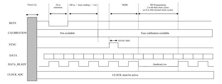
Figure 19. Software reset and start up procedure
