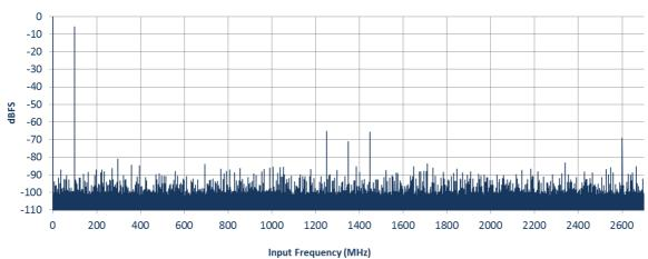
Figure 35. FFT at 5.4GSps and Fin = 1900MHz / -1dBFS
