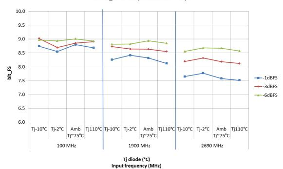
Versus Temperature - Typical supplies - 4 cores interleaved (Staggered mode).
