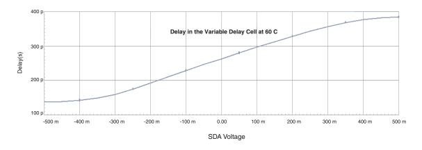
The variation of the delay in function of the temperature is negligible. If this function is not used, SDAEN can be left floating as well as the SDA pin.
