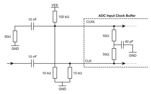
In the case of an application requiring a fixed clock frequency, it is recommended to filter the clock signal for improved jitter performance. The benefits of filtering the clock signal can be quantified to a 1 or 2 dB improvement in the SNR figure and thus in an increase of about 0.1 to 0.2 bit in the ENOB figure.
