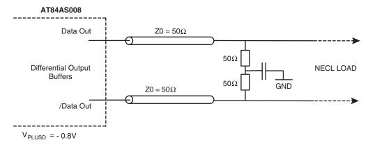
When connected to the AT84CS001 DMUX from e2v, the ADC has to be set in LVDS ( $V_{PLUSD} = 1.45V$ ). The ADC outputs need to be  $100\Omega$  terminated and since the AT84CS001 DMUX input buffers are already on-chip 2 x  $50\Omega$  terminated, the ADC can be connected directly to the DMUX as shown in Figure 3-2.
