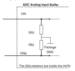
Figure 2-5. AT84AS008 Analog Input Termination Scheme (Differential)
