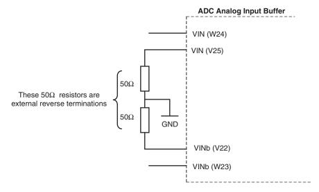
Figure 2-5. AT84AS003 and AT84AS004 Analog Input Termination Scheme (Differential)
