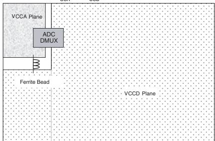
For more information concerning the power supplies decoupling and bypassing, please refer to the device datasheet (reference 0808 and 0829 for the AT84AS003 and AT84AS004 devices respectively).
